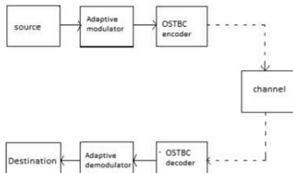
Fig.1 Block Diagram of MIMO System
